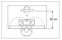
► Position the monitor so that the eye distance to the screen (1) is around 50 cm.
